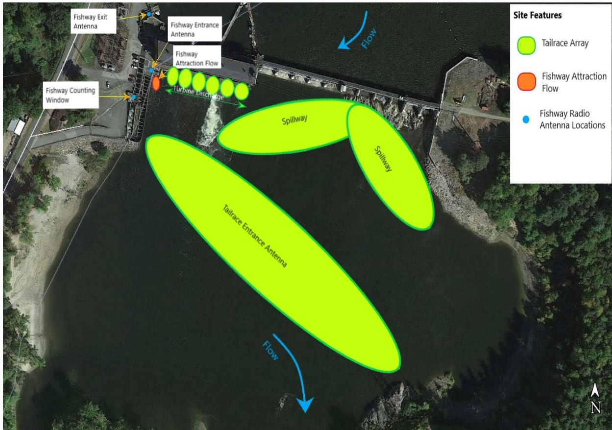
AIR 4, Figure 2. Detection zones for the Vernon tailrace array (tailrace entrance, spillway and turbine discharge antennas) and fishway monitoring stations used in 2015 as part of ILP Study 21 (American Shad Telemetry) and used in this assessment of FirstLight tagged sea lamprey movement at Vernon.
