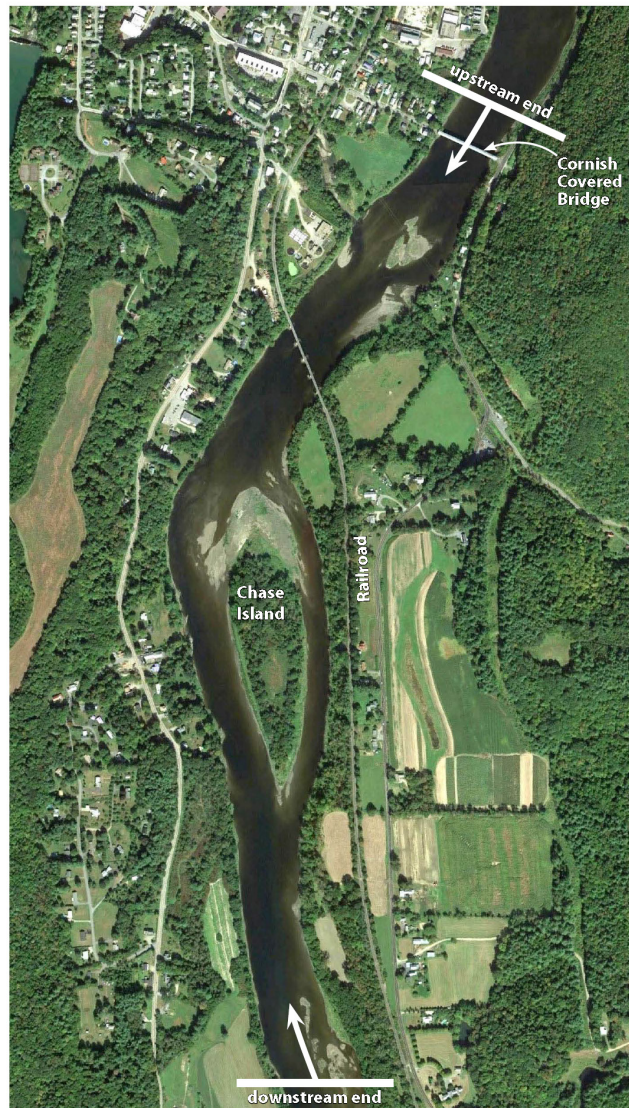
Figure 1. Reach from Cornish Covered Bridge to below Chase Island. This 2,400-meter reach of the Connecticut River at the lower end of the free-flowing reach and upper end of the Bellows Falls impoundment is where quantitative mussel sampling and two-dimensional (2-D) hydrodynamic modeling are proposed to assess and quantify the effects of water-level fluctuations on freshwater mussels and their habitat.
