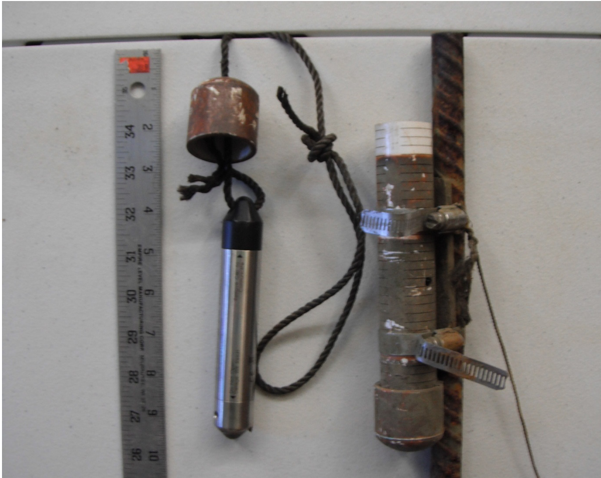
Figure 8-4. Installation set-up used for HOB0 level loggers.
