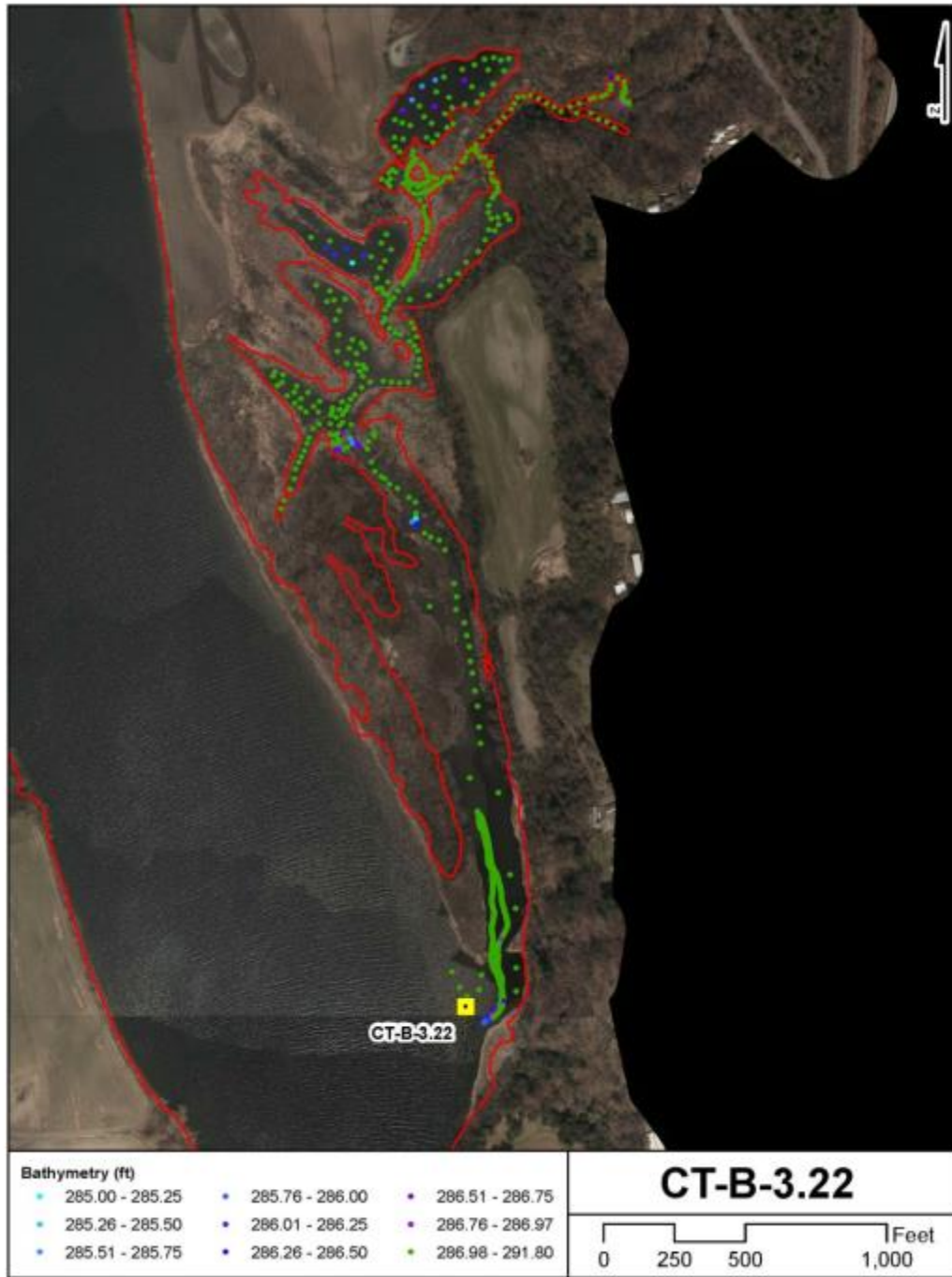
Figure C-16. Plan view of available bathymetry data at tributary site CT-B-3.22 (Clay Brook, Stream Order 4). Color scale is relative to the low water elevation of 286.98' as recorded at level logger station 49 (green = dry, blue-pink = deeper-shallower).
