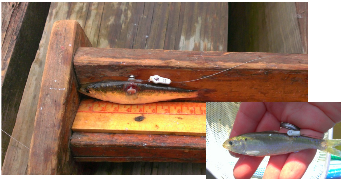
Figure 2-4. Tagging Trial-1, example of tagged juvenile American Shad using Lotek model NTC M-2 transmitter with Hi-Z tag attachment (top); and Lotek model NTQ-1 transmitter with No. 16 dry fly hook as used in Tagging Trial-2 and -3 (inset).
