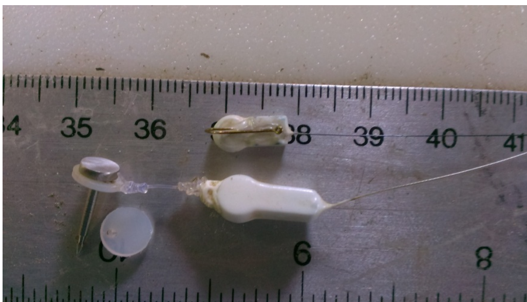
Figure 2-3. Transmitters used for tagging trials. Lotek model NTC M-2 transmitter with Hi-Z tag attachment used in Tagging Trial-1 (bottom); Lotek model NTQ-1 transmitter with No. 16 dry fly hook as used in Tagging Trial-2 and -3 (top).
