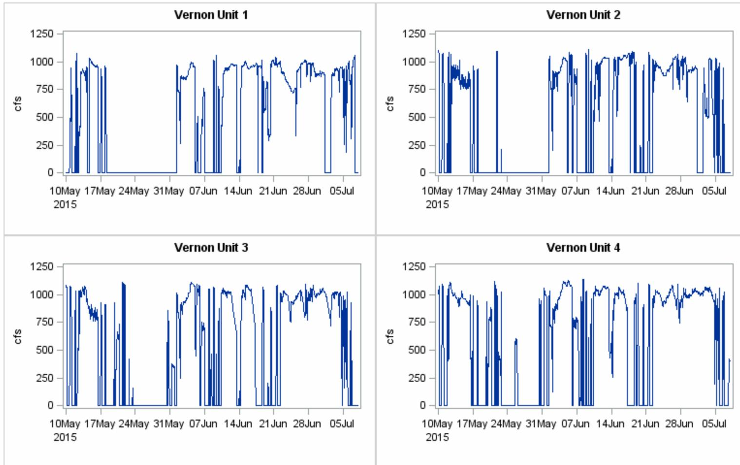
Figure 5.2-2. Hourly discharge for Units 1-4 (133 rpm single runner Francis units) at Vernon during the study period, May 10 – July 7, 2015.
