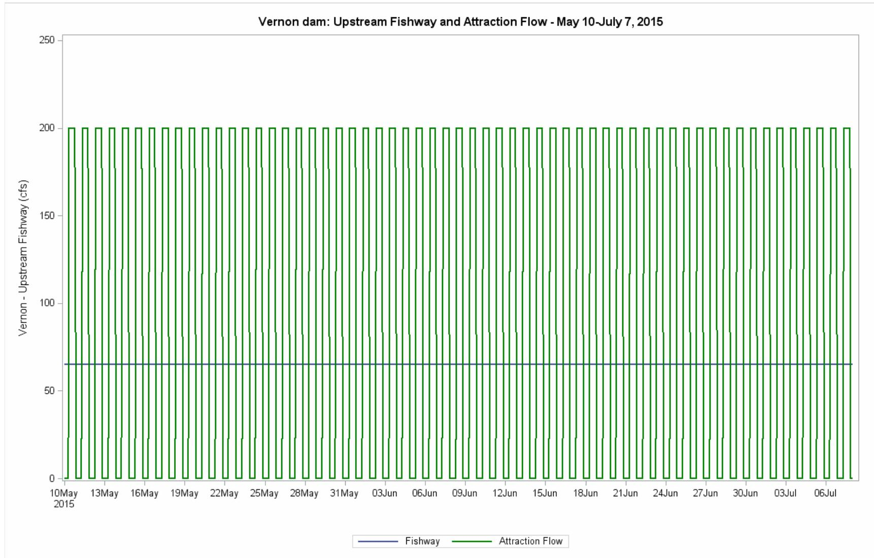
Figure 5.2-6. Upstream fish ladder discharge (cfs) and attraction pump flow (cfs) at Vernon dam during the study period, May 10 – July 7, 2015.
