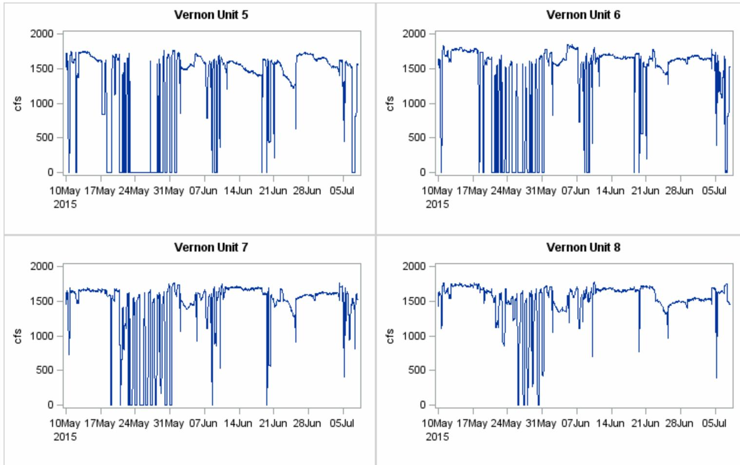
Figure 5.2-3. Hourly discharge for Units 5-8 (144 rpm axial flow Kaplan units) at Vernon during the study period, May 10 – July 7, 2015.
