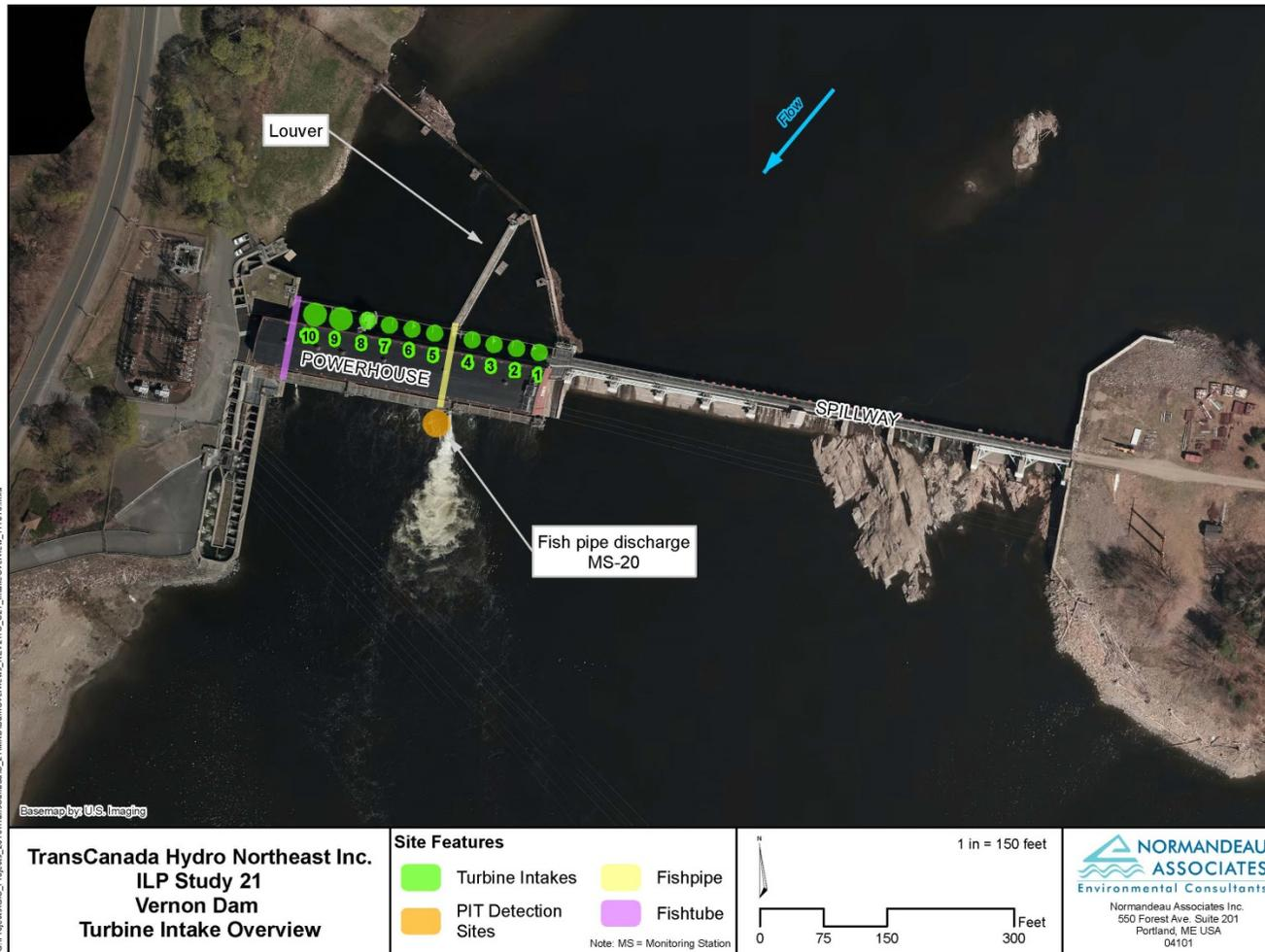
Figure 4.3-4. PIT tag monitoring station on the downstream end of the fish pipe downstream passage route (MS-xx = Monitoring Station xx).
