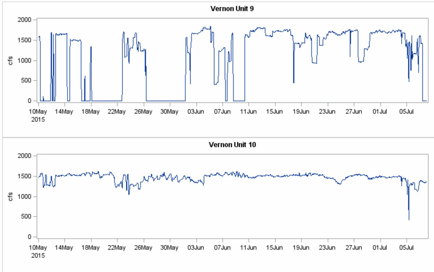
Figure 5.2-4. Hourly discharge for Units 9-10 (75 rpm single runner Francis units) at Vernon during the study period, May 10 – July 7, 2015.
