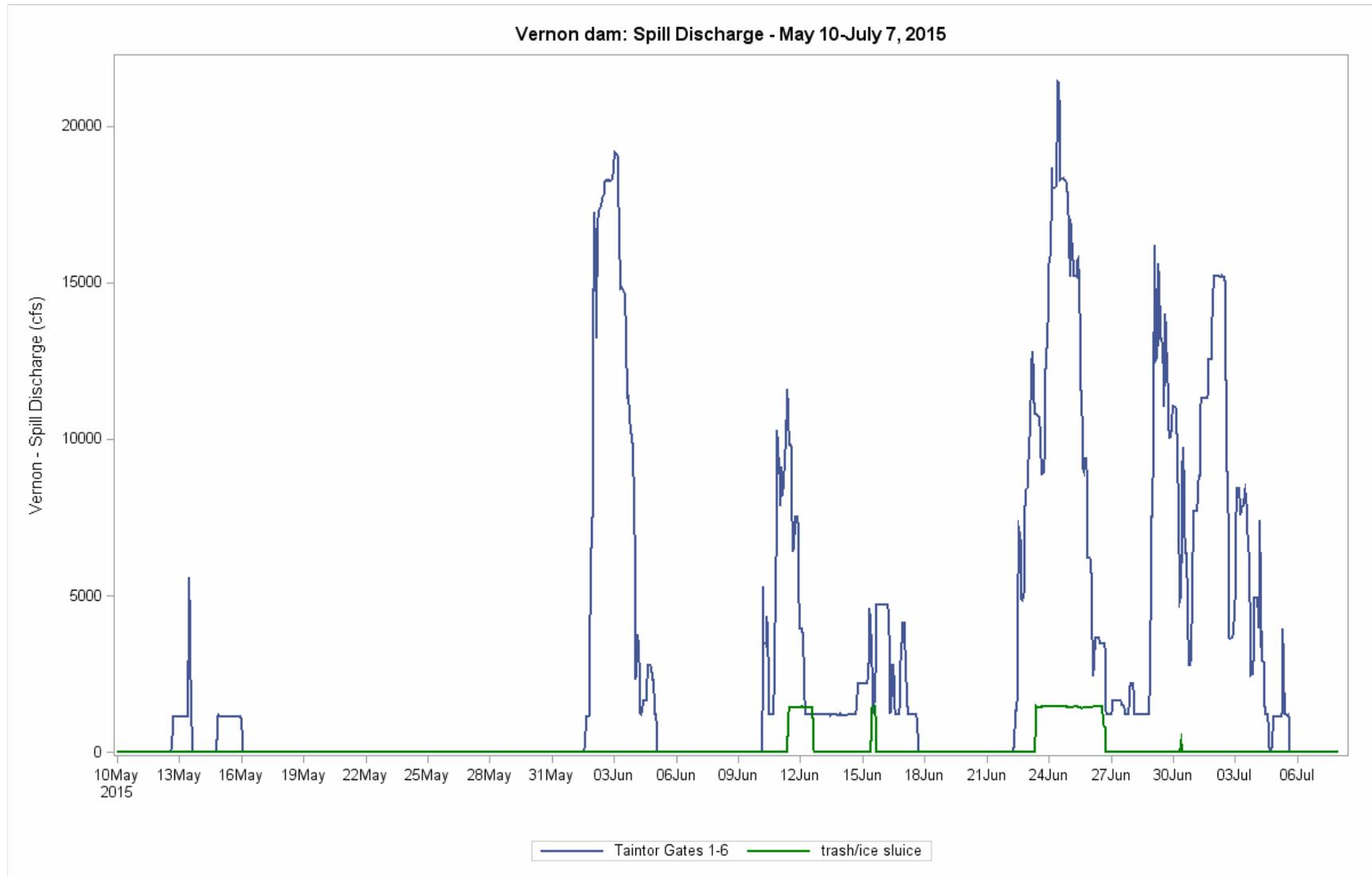
Figure 5.2-5. Spill discharge (cfs) by gate type at Vernon dam during the study period, May 10 – July 7, 2015.
