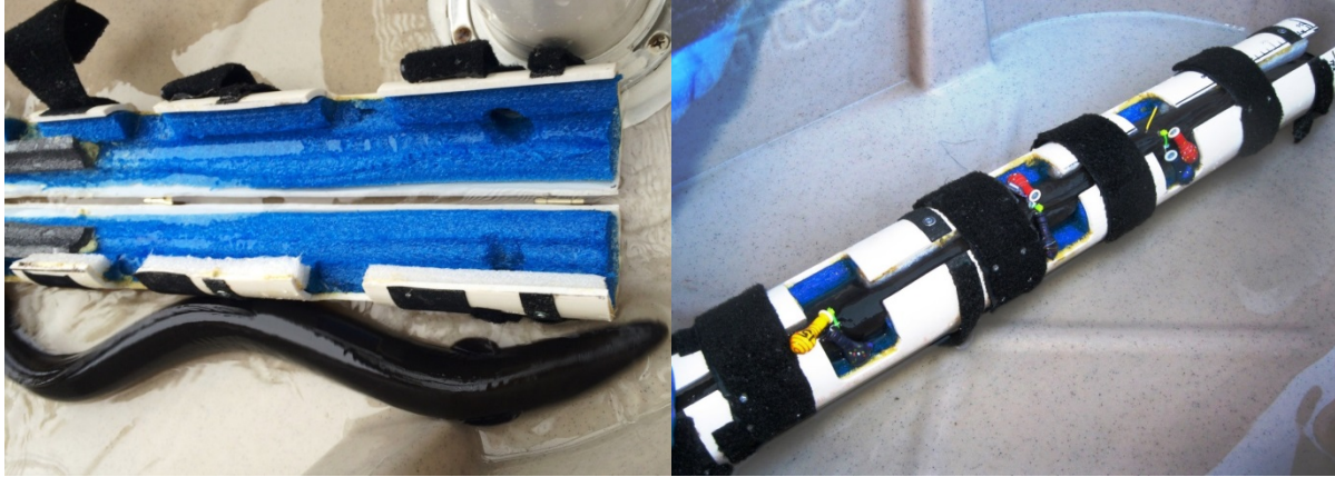
Figure 4.3.3-2. Restraining device used to aid in HI-Z tagging with eel ready for release through the induction system.
