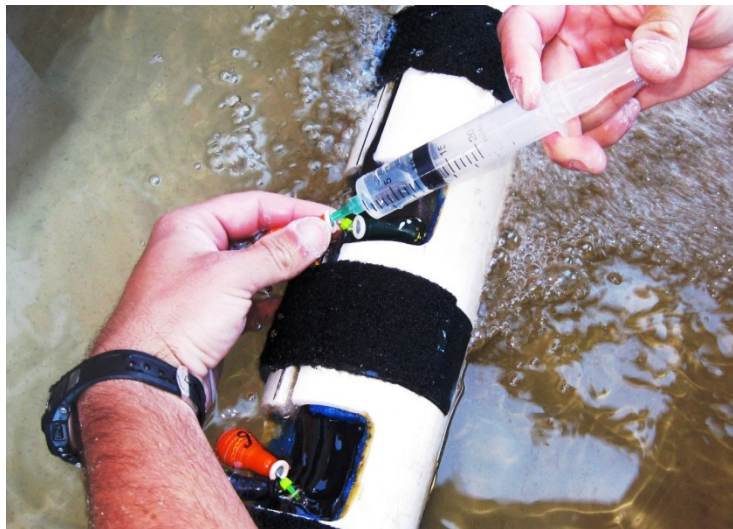
Figure 4.3.3-3: Injecting catalyst into a HI-Z tag attached to an adult American Eel.
