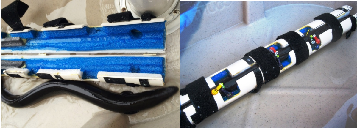
Figure 4.3.3-2. Restraining device used to aid in HI-Z tagging with eel ready for release through the induction system.
