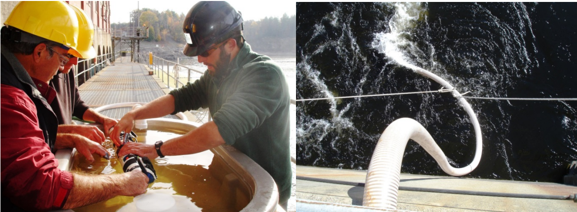
Figure 4.3.3-8. Control induction system and release hose used to release HI-Z tagged adult American Eels.
