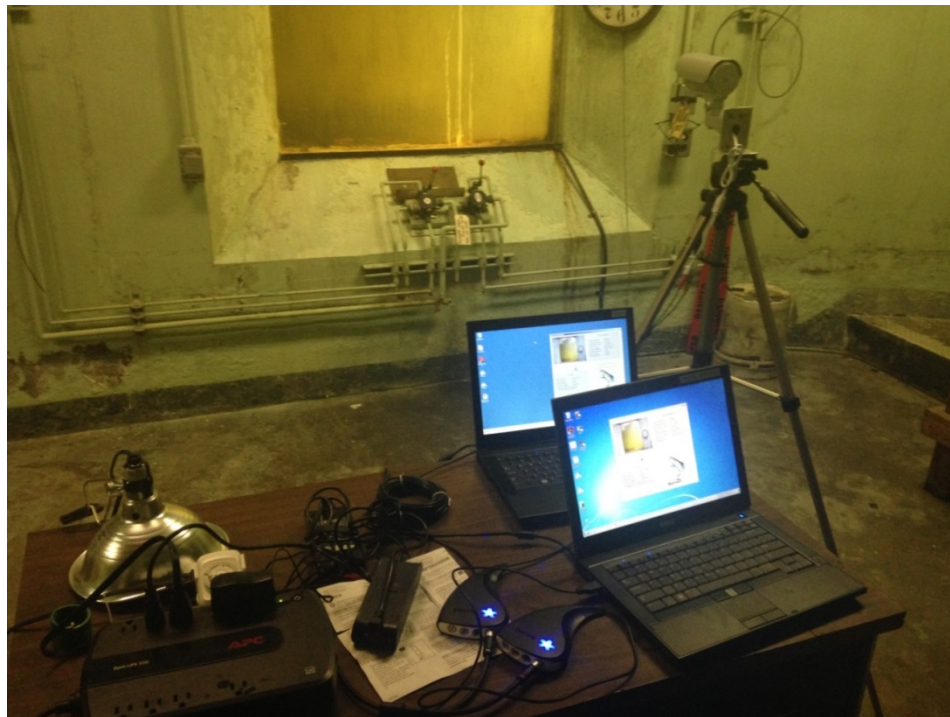
Figure 3.1-1. Salmonsoft FishCap digital video counting system equipment set-up at the Vernon Dam fish ladder with additional laptop for weekly video download and quality control video capture.
