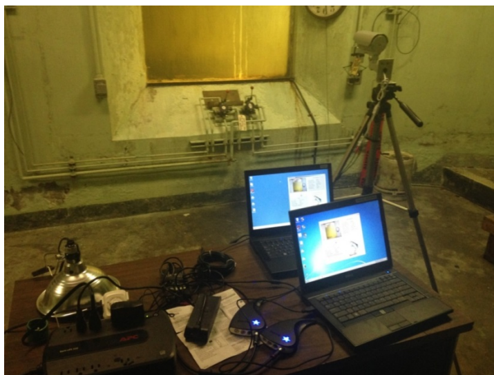
Figure 3.1-1. Salmonsoft FishCap digital video counting system equipment set-up at the Vernon Dam fish ladder with additional laptop for weekly video download and quality control video capture.
