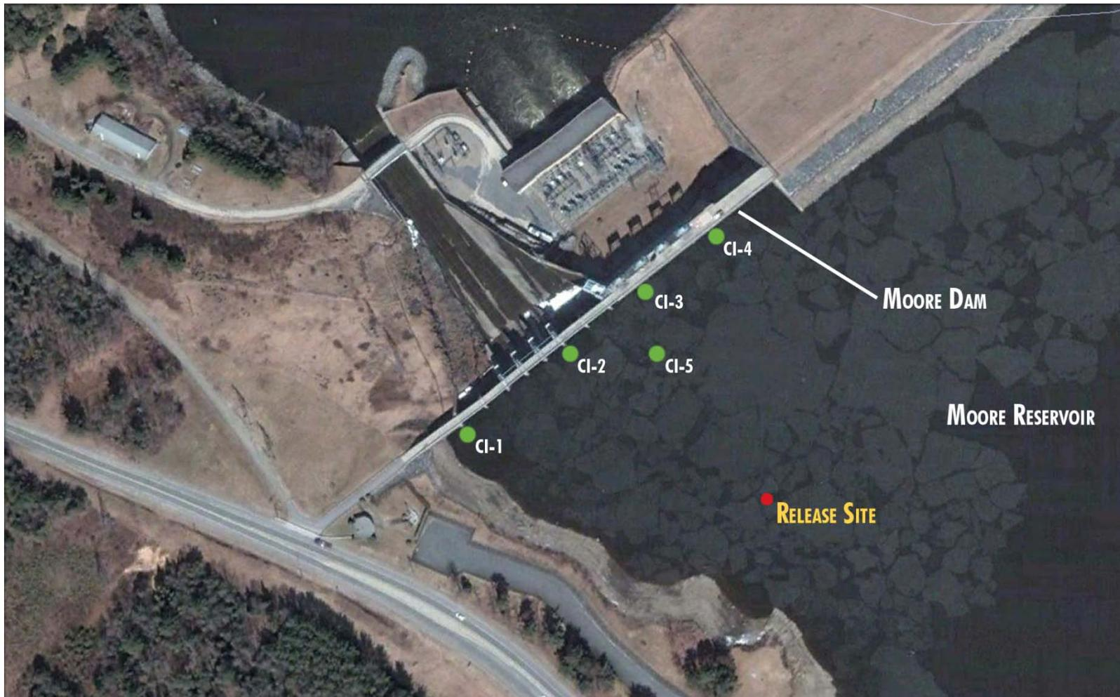
Figure 3-1. Map showing the release site for tagged hatchery fish and the location of five units (CI-1 through CI-5) of a current inducer fish guidance system installed in the Moore Reservoir, spring 2010.
