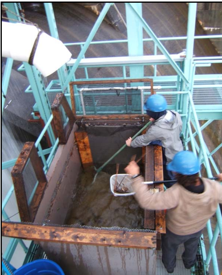
Figure 3-1. Fish collection tank and discharge pipe. The lower end of the sampler screen is raised to curtail flow to the collection tank while the sample is collected.
