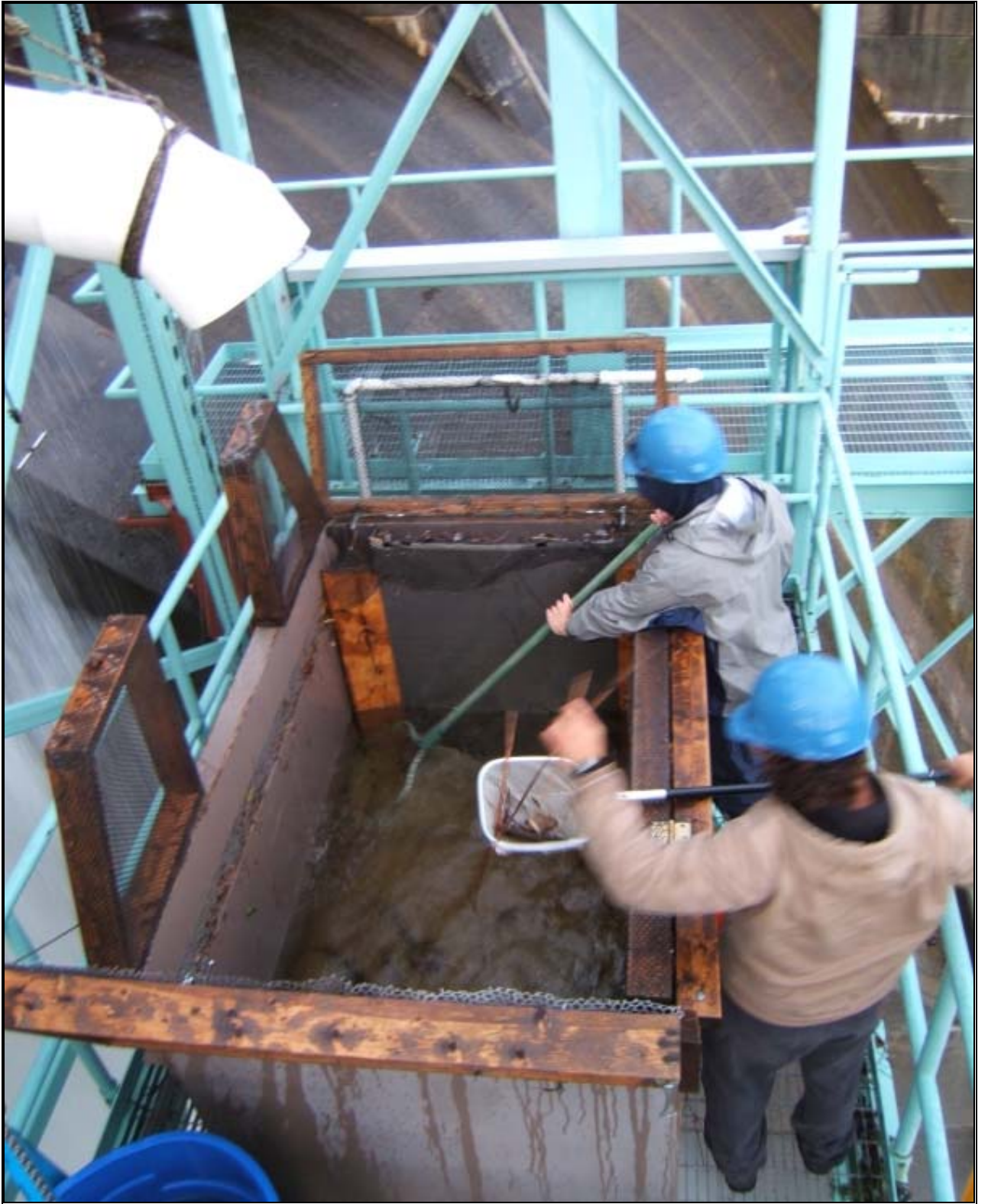
Figure 3-1. Fish collection tank and discharge pipe. The distal end of the sampler is raised to curtail flow to the collection tank while the sample is collected.
