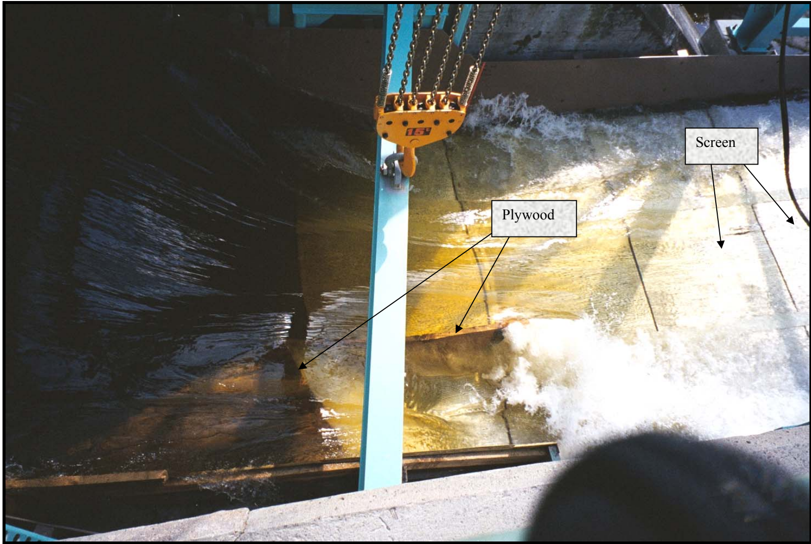
Figure 2-3. Moore Development, inclined plane sampler showing plywood flow adjusters.
