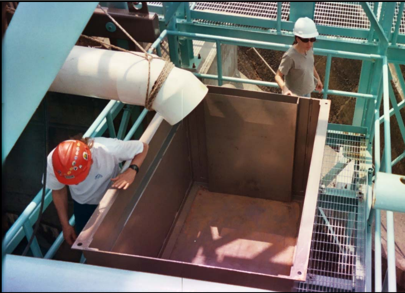
Figure 2-5. Collection tank, located below the inclined plane sampler at USGen NE's Moore Development.
