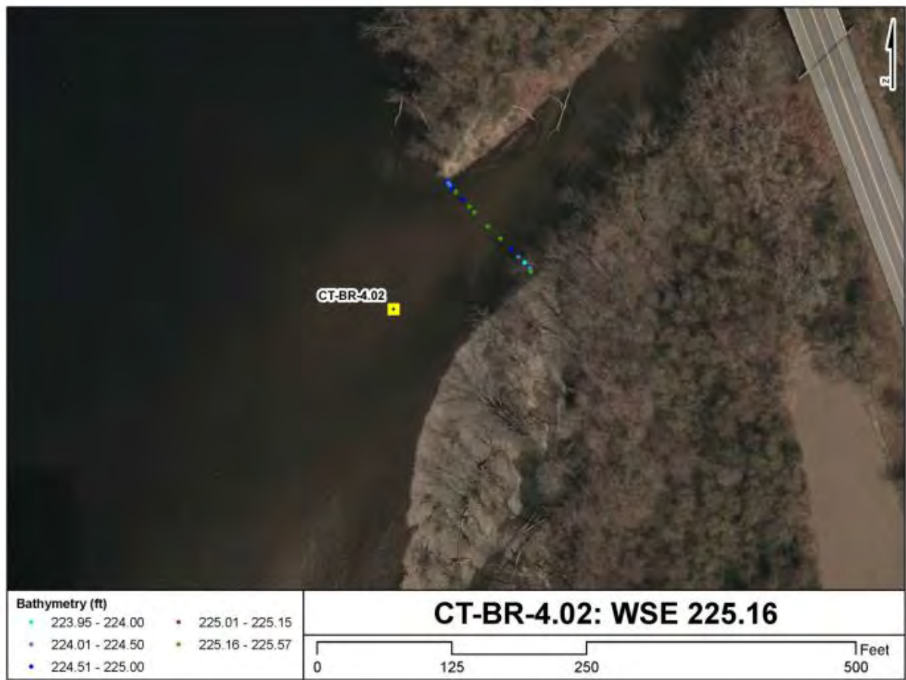
Figure C-20. Plan view of available bathymetry data at tributary site CT-BR-4.02 (Cold River, Stream Order 5). Color scale is relative to the low water elevation of 225.16' observed at the time of sampling (green = dry, blue-pink = deeper-shallower).
