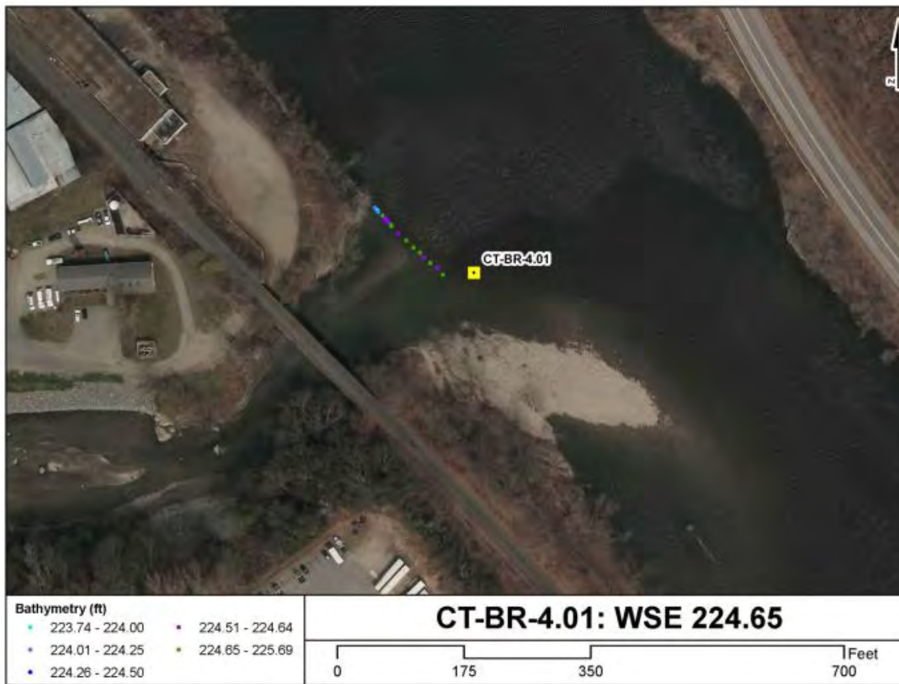
Figure C-19. Plan view of available bathymetry data at tributary site CT-BR-4.01 (Saxtons River, Stream Order 5). Color scale is relative to the low water elevation of 224.65' observed at the time of sampling (green = dry, blue-pink = deeper-shallower).
