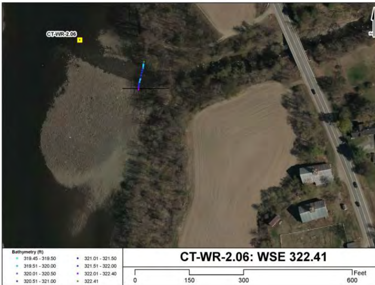
Figure C-7. Plan view of available bathymetry data at tributary site CT-WR-2.06 (Bloods Brook, Stream Order 4). Color scale is relative to the low water elevation of 322.41' observed at the time of sampling (green = dry, blue-pink = deeper-shallower).
