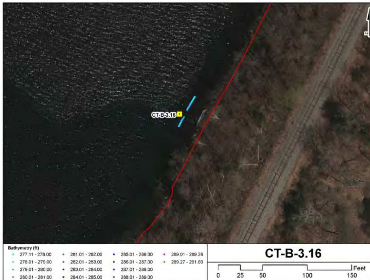
Figure C-13. Plan view of available bathymetry data at tributary site CT-B-3.16 (Beaver Brook, Stream Order 4). Color scale is relative to the low water elevation of 289.27' as recorded at level logger station 43 (green = dry, blue-pink = deeper-shallower).
