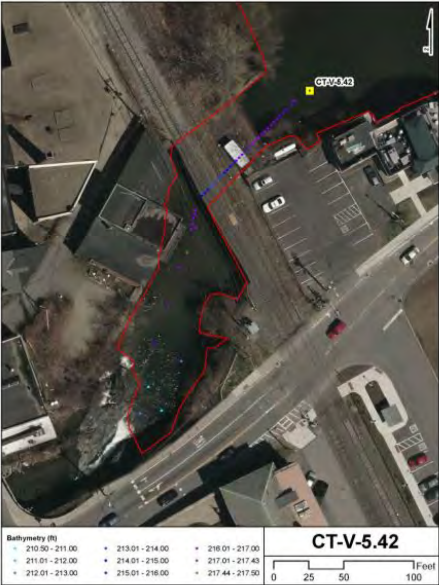
Figure C-27. Plan view of available bathymetry data at tributary site CT-V-5.42 (Whetstone Brook, Stream Order 4). Color scale is relative to the low water elevation of 217.44' as recorded at level logger station 65 (green = dry, blue-pink = deeper-shallower).
