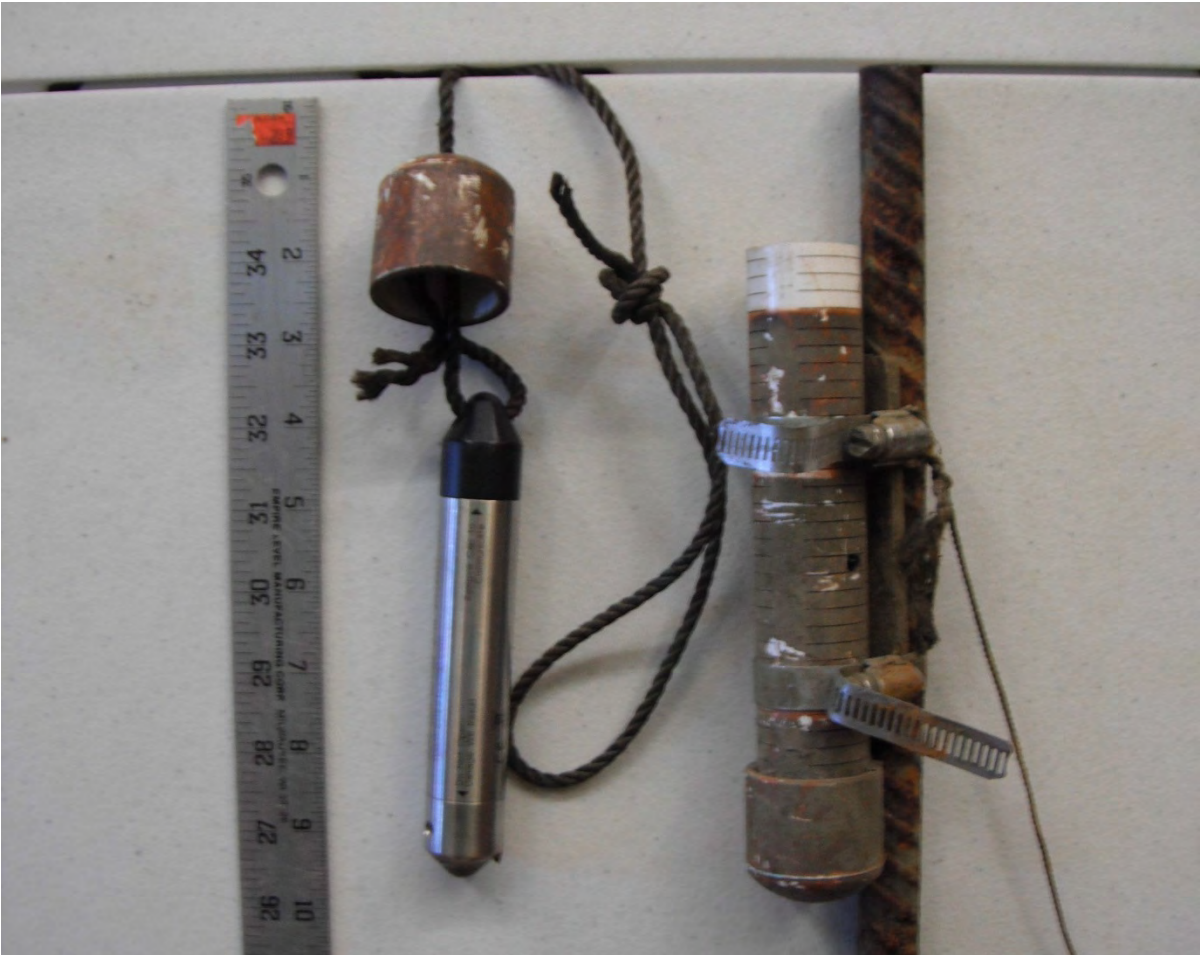
Figure 8-4. Installation set-up used for HOB0 level loggers.
