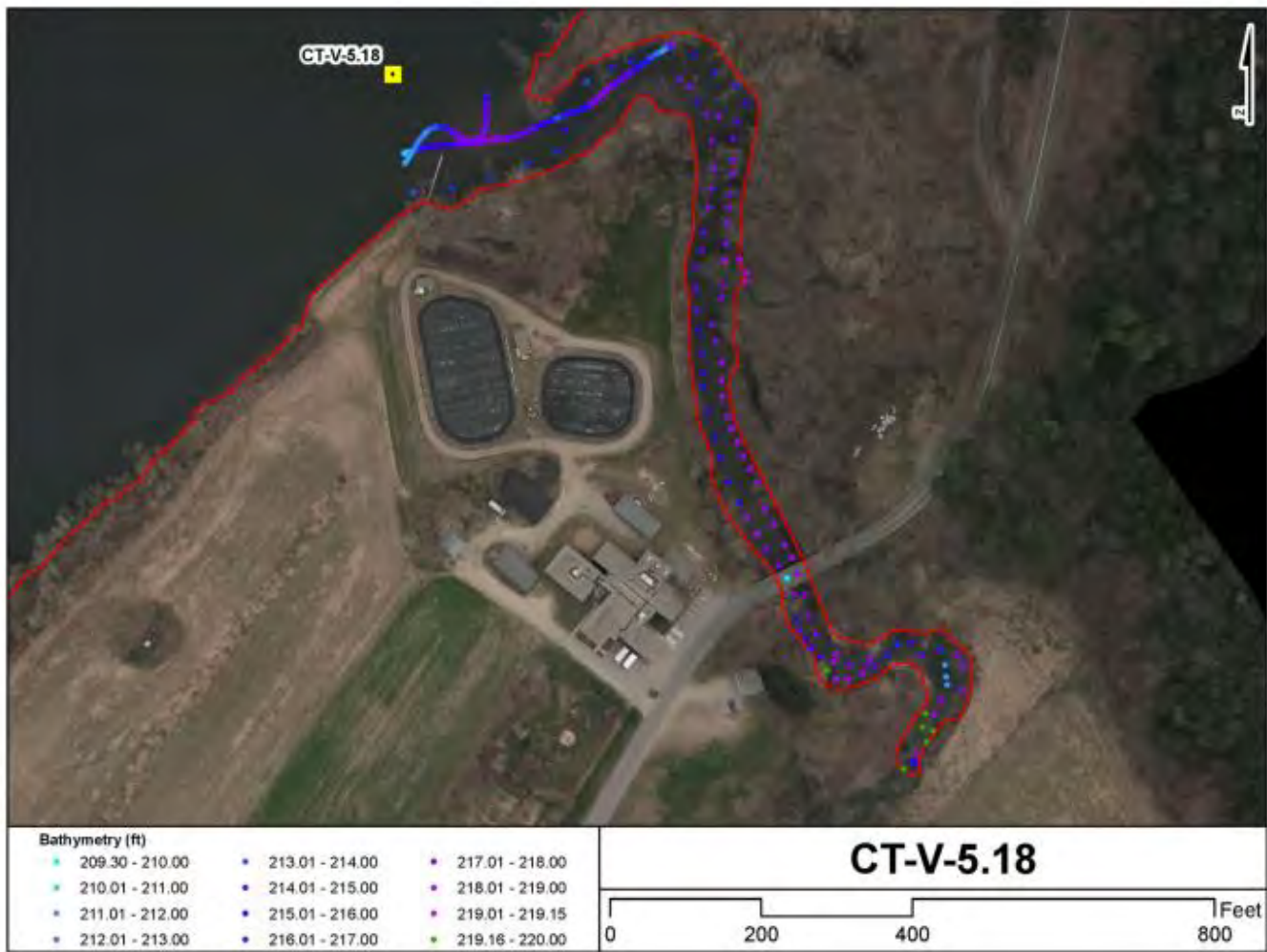
Figure C-23. Plan view of available bathymetry data at tributary site CT-V-5.18 (Partridge Brook, Stream Order 4). Color scale is relative to the low water elevation of 219.16' as recorded at level logger station 60 (green = dry, blue-pink = deeper-shallower).
