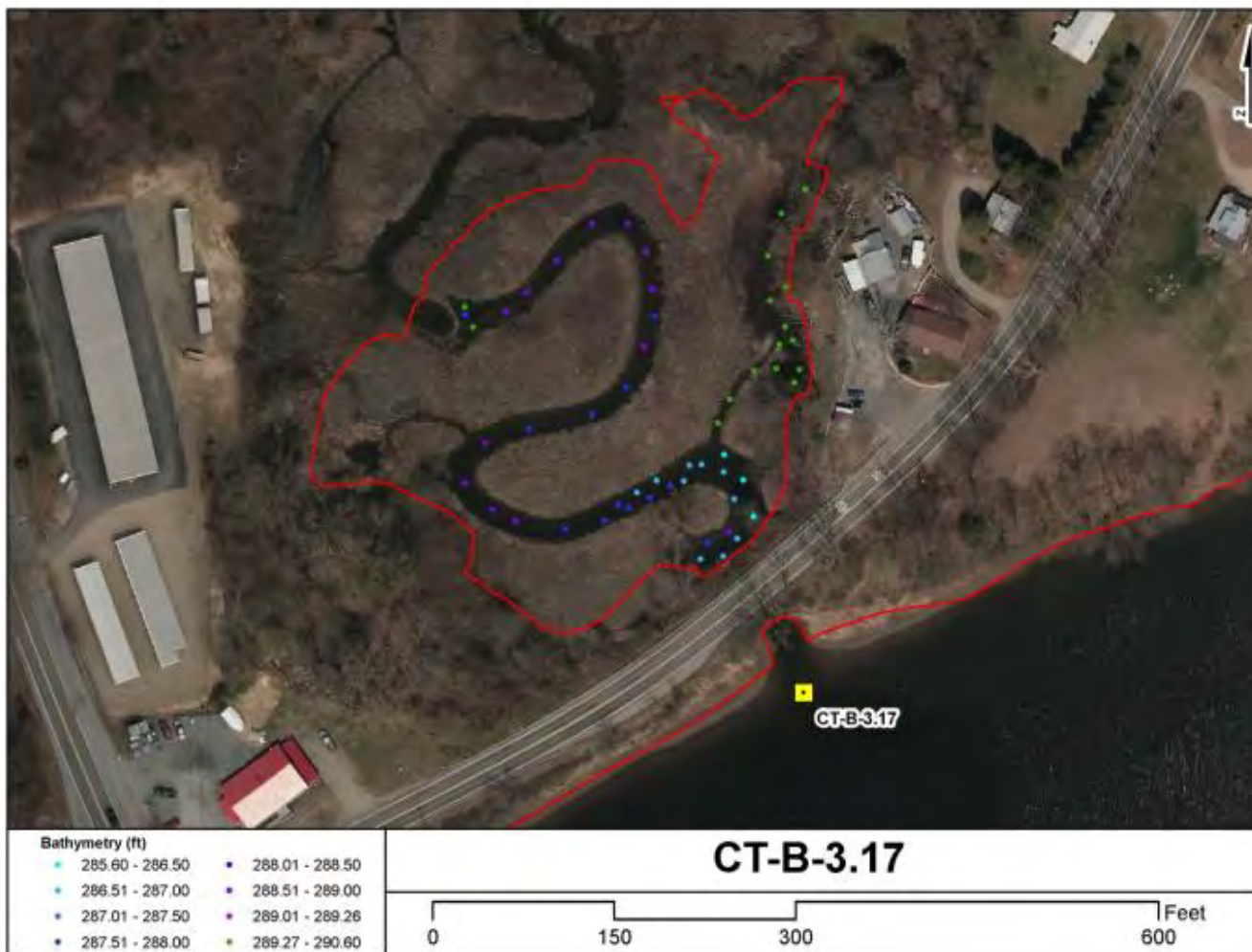
Figure C-14. Plan view of available bathymetry data at tributary site CT-B-3.17 (Spencer Brook, Stream Order 4). Color scale is relative to the low water elevation of 289.27' as recorded at level logger station 43 (green = dry, blue-pink = deeper-shallower).
