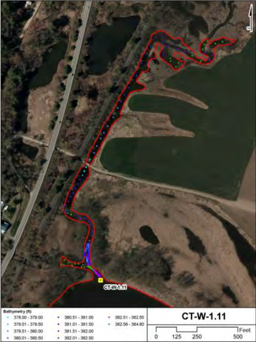
Figure C-2. Plan view of available bathymetry data at tributary site CT-W-1.11 (Halls Brook, Stream Order 4). Color scale is relative to the low water elevation of 382.56' as recorded at level logger station 5 (green = dry, blue-pink = deeper-shallower).
