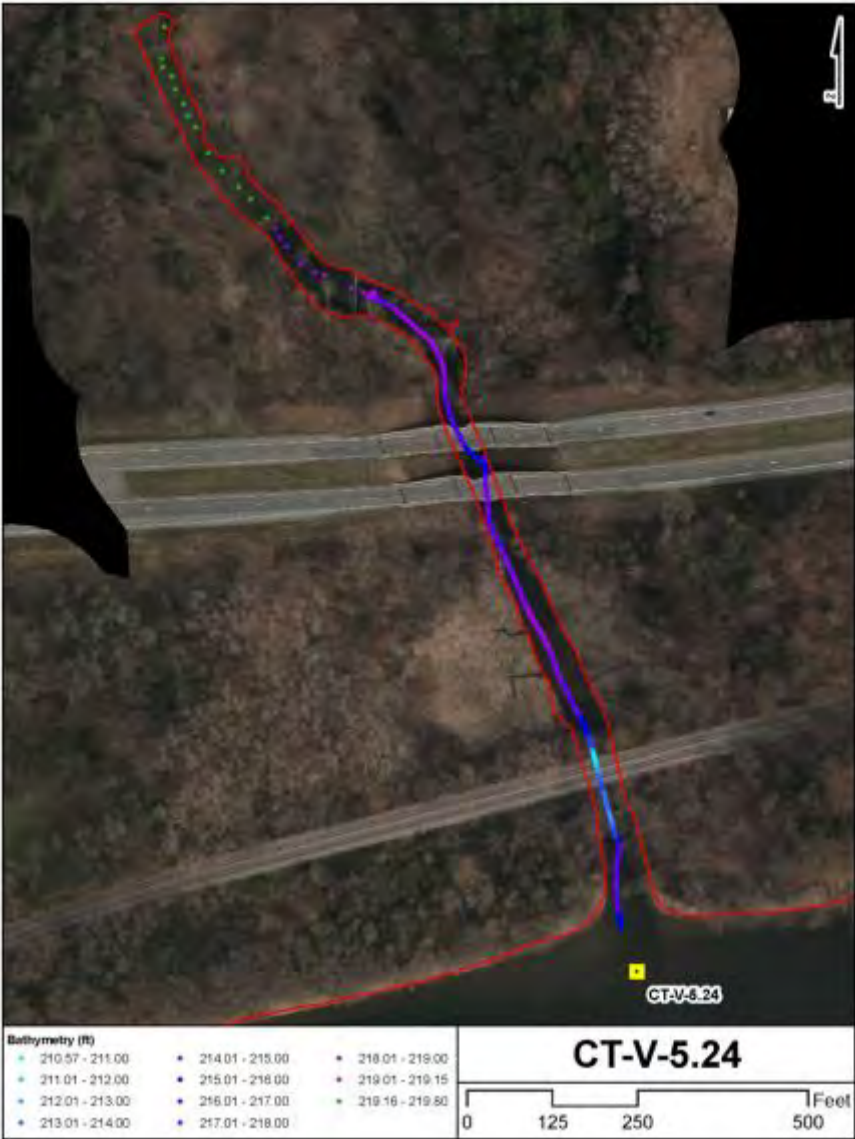
Figure C-25. Plan view of available bathymetry data at tributary site CT-V-5.24 (Sacketts Brook, Stream Order 4). Color scale is relative to the low water elevation of 219.16' as recorded at level logger station 60 (green = dry, blue-pink = deeper-shallower).
