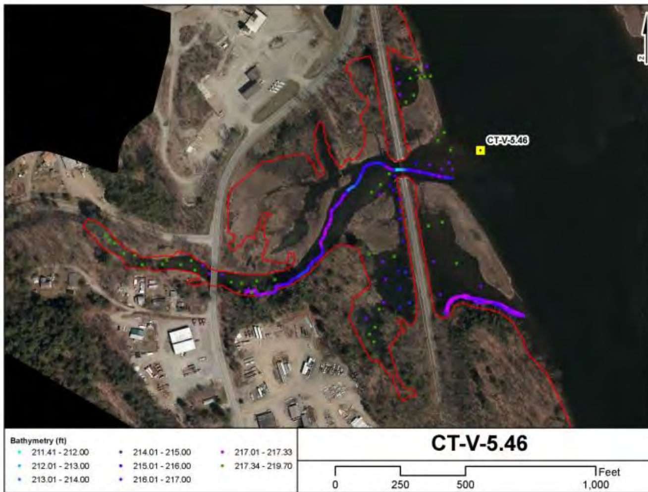
Figure C-28. Plan view of available bathymetry data at tributary site CT-V-5.46 (Broad Brook, Stream Order 4). Color scale is relative to the low water elevation of 217.34' as recorded at level logger station 70 (green = dry, blue-pink = deeper-shallower).
