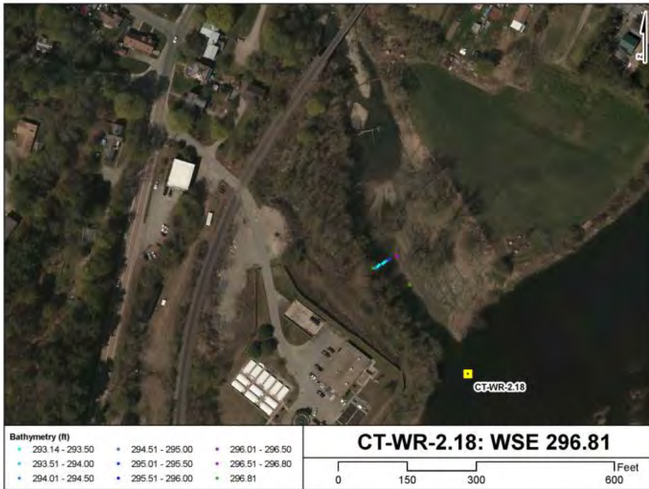
Figure C-9. Plan view of available bathymetry data at tributary site CT-WR-2.18 (Mill Brook (VT), Stream Order 4). Color scale is relative to the low water elevation of 296.81' observed at the time of sampling (green = dry, blue-pink = deeper-shallower).
