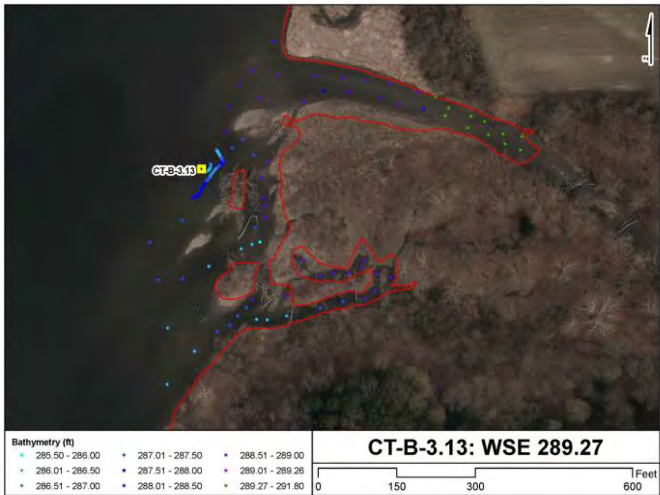
Figure C-12. Plan view of available bathymetry data at tributary site CT-B-3.13 (Little Sugar River, Stream Order 4). Color scale is relative to the low water elevation of 289.27' as recorded at level logger station 43 (green = dry, blue-pink = deeper-shallower).
