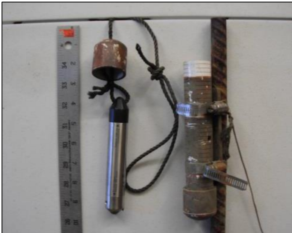
Figure 4.3-2. Installation set-up used for HOBO water level loggers.
