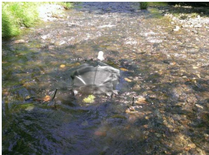
Figure 5.3-2. Sea Lamprey nest cap, Partridge Brook (site 16-VT-018-B).
