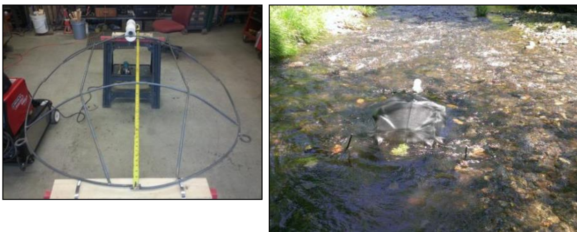
Figure 4.3-1. Sea Lamprey nest cap: frame (left panel) and deployed in the field (right panel).
