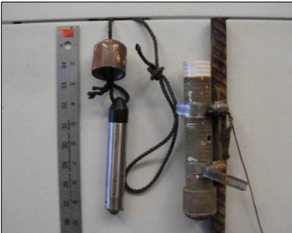
Figure 4.3-2. Installation set-up used for HOBOWare water level loggers.
