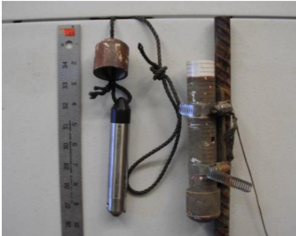
Figure 4.1-1. Installation set-up used for HOBOWare water level loggers.
