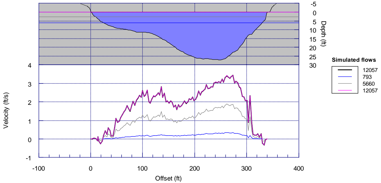
Cross-section: WR1-6 Pool: Manning Ns applied IFG4 method
