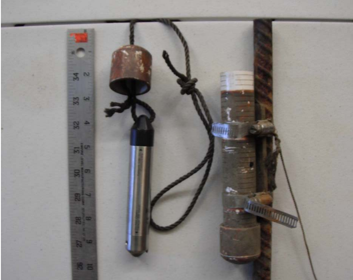
Figure 8-4. Installation set-up used for HOB0 level loggers.
