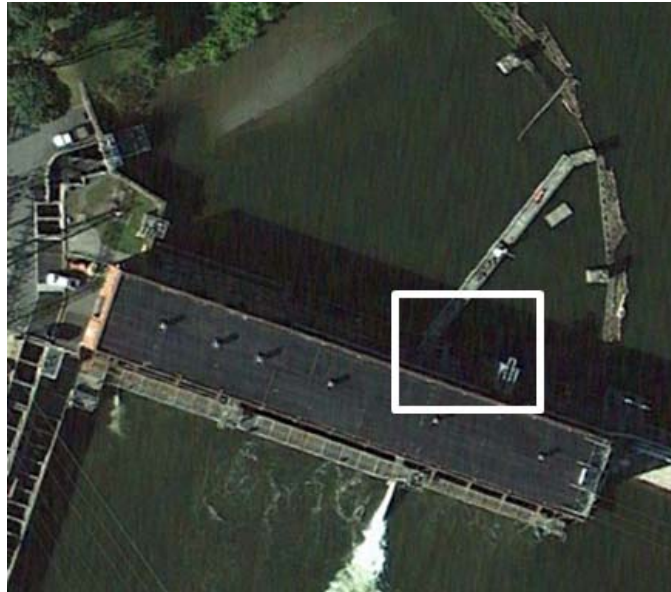
Figure A-1. Conceptual diagram of the location of a single split-beam transducer (in white square) mounted to sample about 100% of the fish pipe entrance for monitoring the temporal pattern in relative abundance of out-migrating juvenile American shad at Vernon dam.
