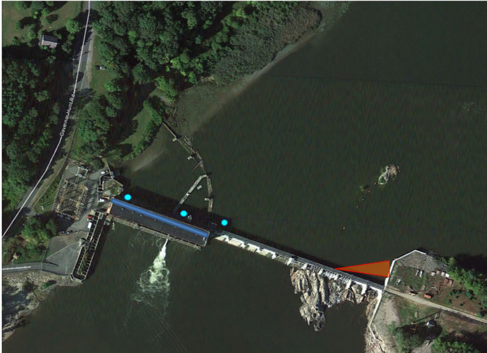
Figure B-2. Conceptual diagram of the dam sampling configuration for Plan B. Cyan dots represent the upward-looking split-beam transducers; Red triangle represent the conical beams of four horizontally aimed transducers pointing across the opening to the two tainter gates; and blue bar representing the bank of 10 upward-looking elliptical split-beam transducers mounted behind the trash racks.
