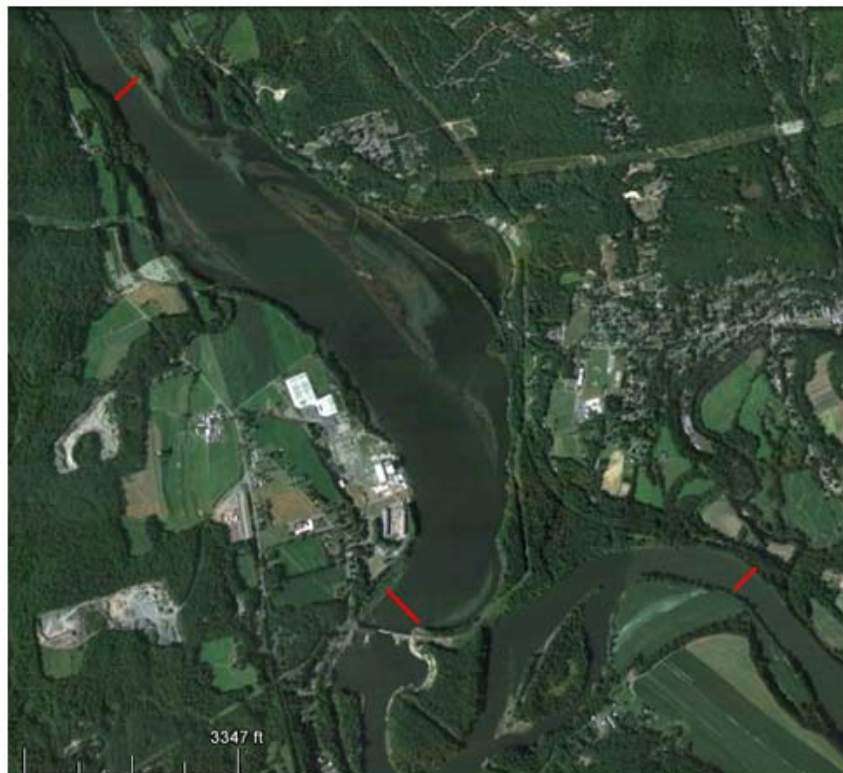
Figure B-1. Conceptual diagram of locations for the three river arrays for Plan B. Red lines mark the upstream, forebay and downstream transducer arrays. Exact locations may change following site evaluations.
