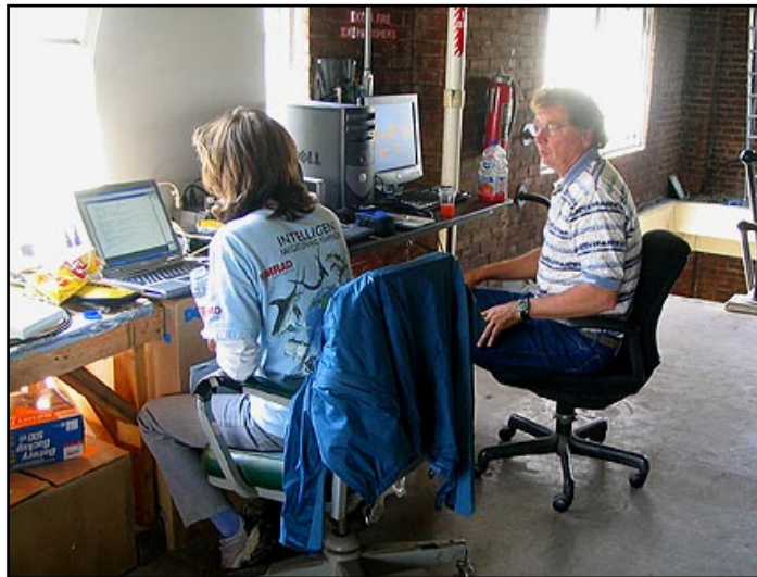
Photo 2. A laptop computer, wireless link, and remote internet system in the Anson powerhouse allowed for local and/or remote operation and monitoring of the hydroacoustic system.
