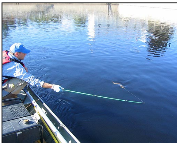
Photo 3. View of a tethered American eel being drifted into position in the hydroacoustic fields.
